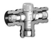
The supplied tempering valves come preset at 50, but can be set at between 40 and 50 degrees by removing the yellow cap and rotating the brass bolt beneath it.
