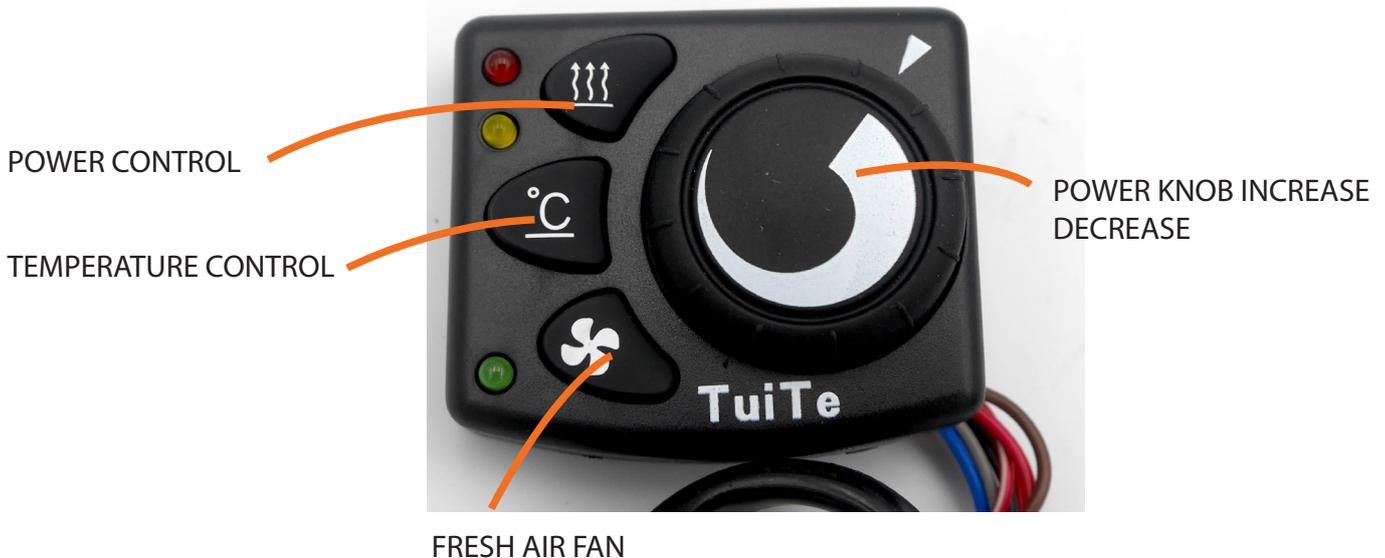
In **Power Control** the heater runs at a constant power level and will not cycle on and off and will remain in constant heat mode, this mode is a lot kinder on power usage. Press the button to turn on, red light will illuminate and the heater will start.
