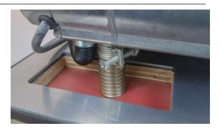
Tip: If the DH12 water service is mounted inside the vehicle the compartment can be covered in 10mm closed cell insulation foam to reduce radiated heat and noise.
