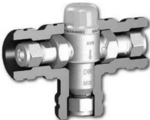
The supplied tempering valves come pre-set at 50, but can be set at between 40 and 50 degrees by removing the yellow cap and rotating the brass bolt beneath it.
