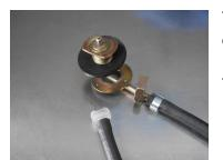
The breather tube fits onto the straw and is clamped down with an ear clamp.
