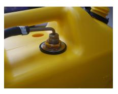
Before installing the fuel straws, shake out any material that might have fallen into the tank from the drilling process.
