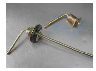
We use a belt sander to cut the fuel straws to length, but an angle grinder can also work.
