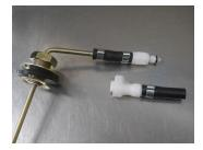
Each end of the quick disconnect is secured using ear clamps.
