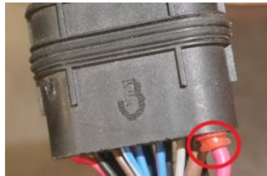
Image 3 and 4. Example of poor connection caused by pin pushed back.
