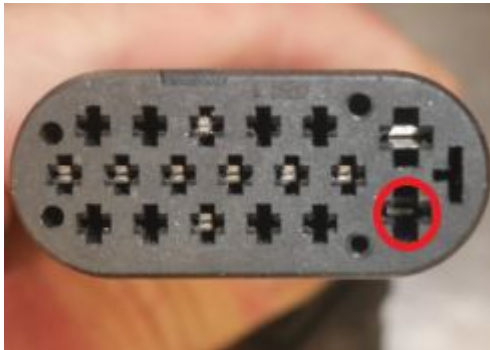
Image 3 and 4. Example of poor connection caused by pin pushed back.
