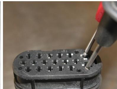
Image 5, 6 and 7. 2kw heater main loom plug with main supply wires identified.
