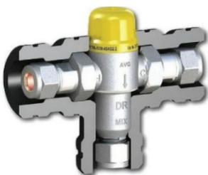
The tempering valves built onto the DH Hydronic hot water heaters come preset at 50°C, but can be set at between 40°C and 55°C by removing the yellow cap and rotating the brass bolt beneath it.
