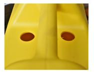
The holes are drilled into the jerry can using a step drill bit.
