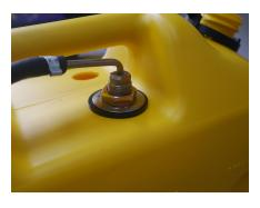
Before installing the fuel straws, shake out any material that might have fallen into the tank from the drilling process.
