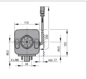
1 Minimum installation distance (clearance) for opening the cover and for dismantling the glow plug and the control box.
