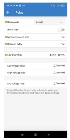
The relay setting for the BMV-712 in the Victron Connect App can be set as shown in the image to allow the system to heat the hot water when the batteries hit 99% and to cut out when they drop to 95%. Depending on your batteries and solar, you may wish to vary the turn off point. However, it is suggested to keep it quite high to minimise 'working' the batteries as the system cycles.
