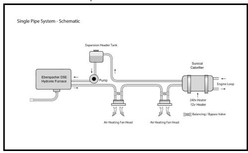
Larger systems have double or parallel pipes and each hydronic item sits across the pipes in parallel. Each item needs its one flow control valve to allow balance of the entire system.
