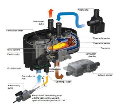
The diesel furnace pumps engine coolant through a closed loop using its own supplied pump. The system is filled via a header tank, which allows for thermal expansion of the coolant and for bleeding out any air. The header tank always has to be located at the highest point in the system.
