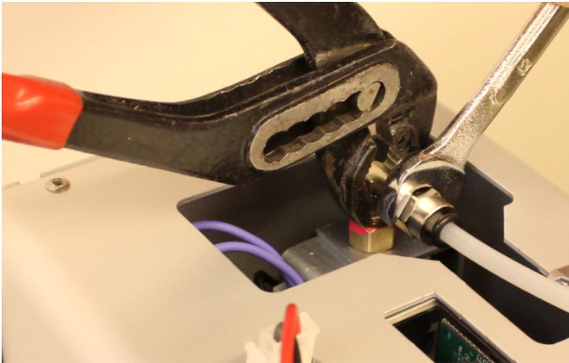
Use pliers to hold the pump inlet elbow steady, while you tighten the 12 mm fuel line nut. The joint has to be very tight to prevent air leaks.
