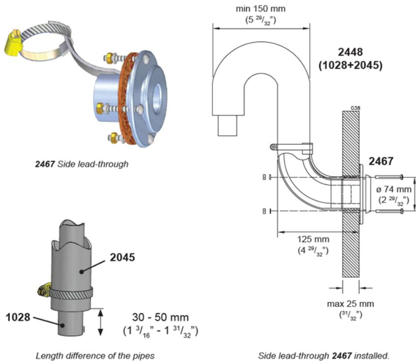
Side lead-through **2467** installed.
