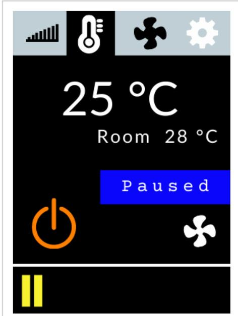
If the heater is in Pause Mode, *Paused* will appear on the screen. Heater will re-start heating again automatically, if the cabin temperature falls 2 degrees C (3,6 F°) below the set target temperature.
