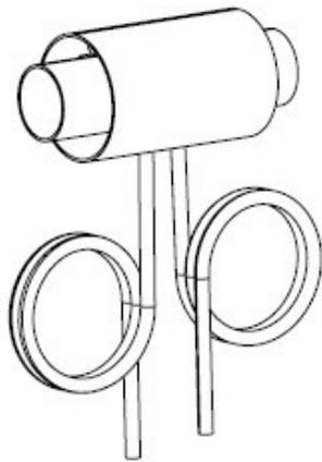
It is recommended that a drainage lock is installed if there is a risk of condensed or splash water entering the exhaust. If necessary, a drainage lock can be installed into the exhaust pipe of a hull lead-through, but note the drainage lock must be positioned after the gooseneck.
