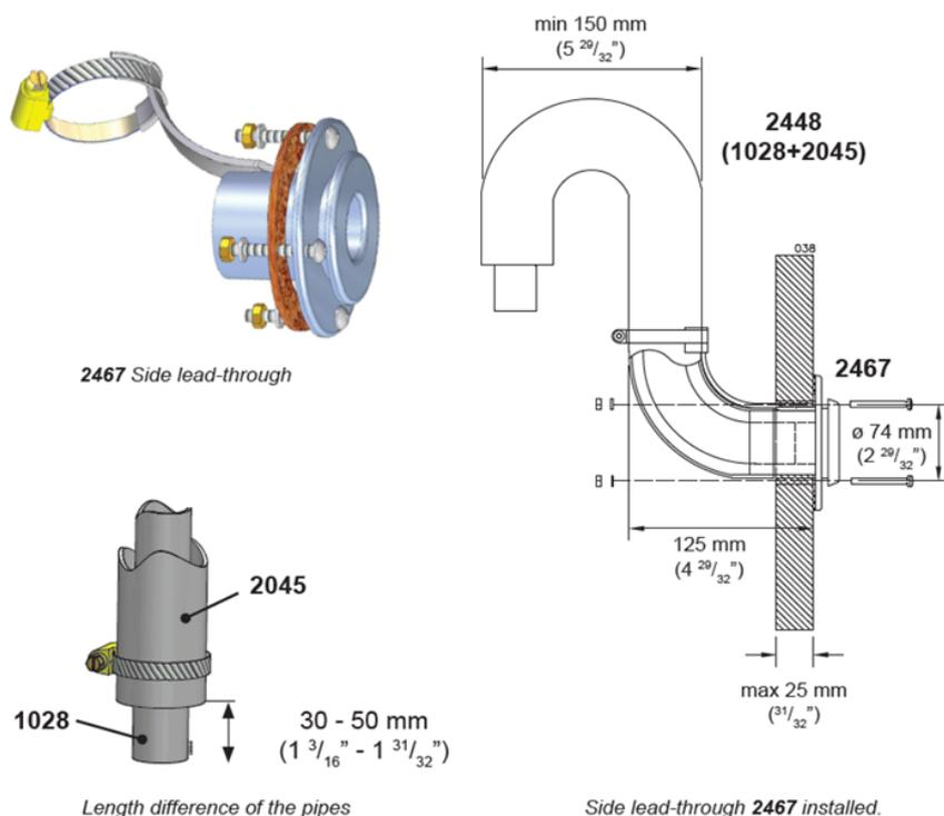
Side lead-through **2467** installed.
