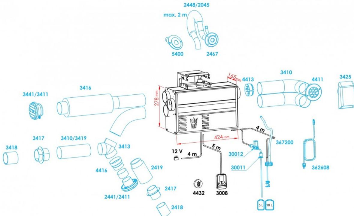
Standard delivery includes Diesel heater, Fuel hose (4m), Power cable (4m), mounting plate, control panel (3008), wired thermo sensor (362608) and wireless temperature beacon (4432).
