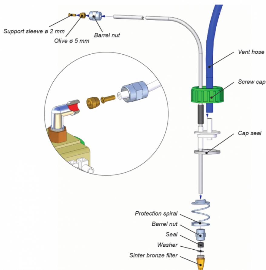
If the fuel will be taken from a separate Wallas day tank, you must install a tank connection **367200** (4 m).
