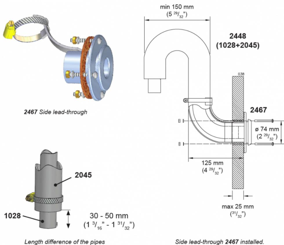
*Side lead-through 2467 installed.
