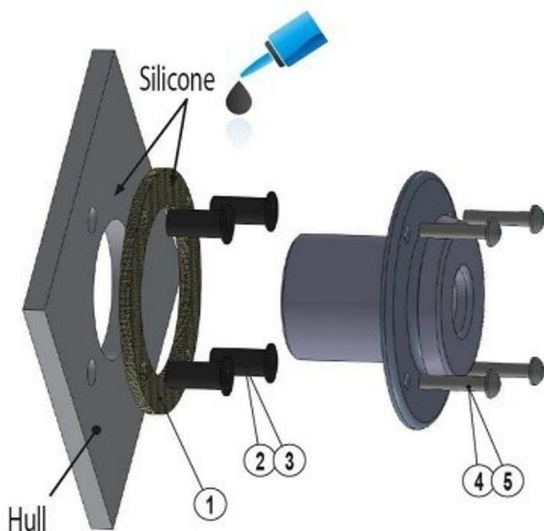
An insulation kit (**2461**) must be used to insulate the lead-through from the boats metal hull. The insulation kit insulates the exhaust gas lead-through and the device from each other. In fault situations the insulation kit prevents electric circuit running between the metal hull and the device. This could result the oxidation or malfunctioning of the devices circuit board and the circuit board would be damaged.
