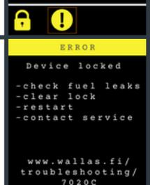
To remove the lock, press any button to return to the main display. Move the selection square to the **Main Menu Bar** and press the **Select Button**, choose **Settings**, and press the **Select Button**. Choose **Clear Lock** from the Settings Menu and press the **Select Button**.
