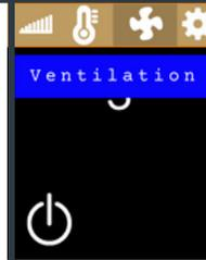
Move the selection square to the **Start/Stop Icon** and press the **Select Button** once. Press the **Select Button** down again for 3 seconds to confirm and start the heater. Yellow Power On light will appear in the Info Bar.
